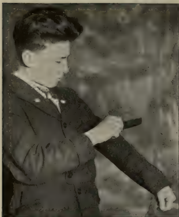
FIG. 109. When the comb is rubbed on the coat, it becomes charged with electricity.
